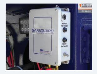
Designed specifically for propane, anhydrous ammonia and butane transports. DCE certified to meet or exceed all US DOT CFR49 and Transport Canada B620-14 regulations. These systems continually monitor the off-loading process, looking for a rapid change in discharge pressure. These systems detect a separated hose or failed connection and close the tank internal valve within 1/2 second.
