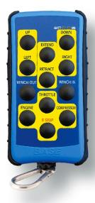
The Ranger handheld can be equipped with different radio technologies depending on your application requirements. Currently three (3) radio technologies are available: Direct Sequence (DSS), Frequency-Hopping Spread-Spectrum (FHS), and Amplitude Shift Keying (ASK).
